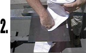
Hold bag just below snap ring while pushing through being careful not to scrape the bag.
