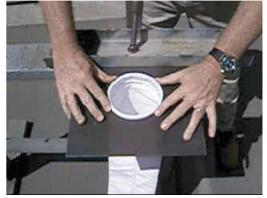
Make sure the seal is even and the bag does not spin within the cell plate.
